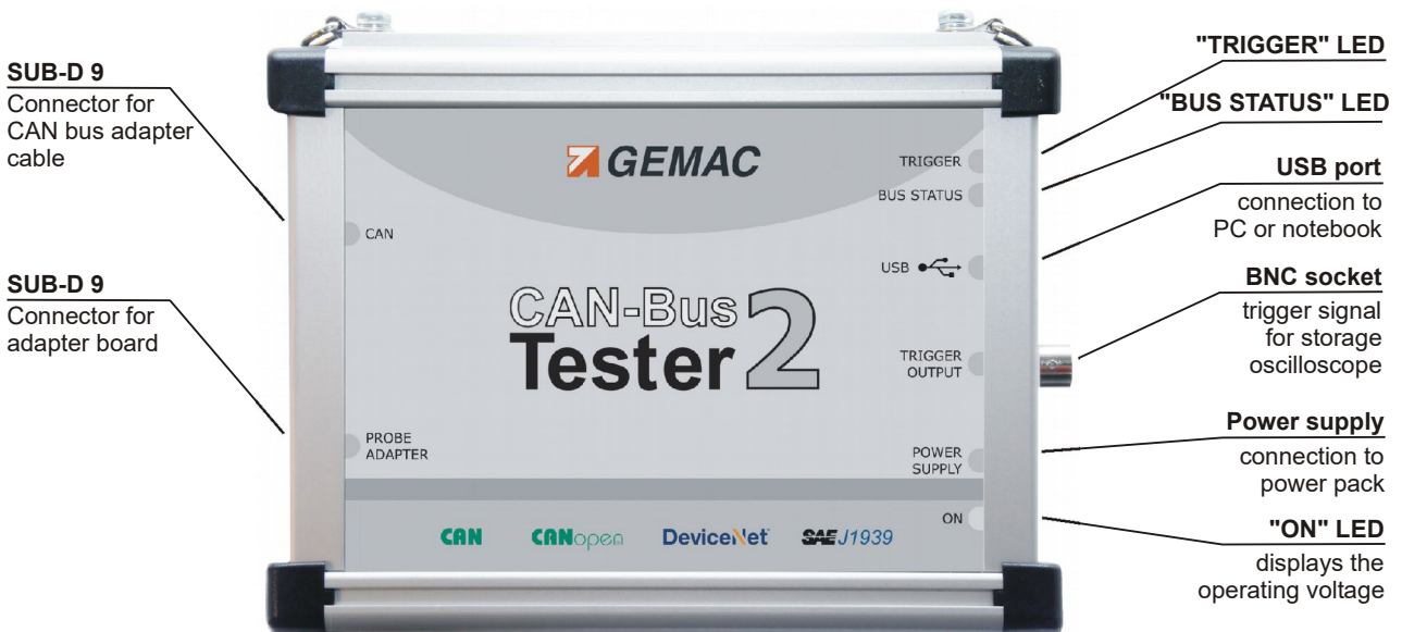
Figure 1: Connections of the CBT2
